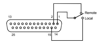
Figure 2–7 Using Local/Remote Operation with Contact Closure
