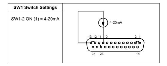
Set up for 4-20 mA programming of the output current as follows:
