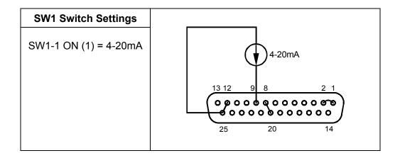
Set up for 4-20 mA programming of the output voltage as follows:
