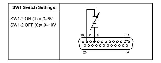
Set up for voltage source programming of the output voltage as follows:
