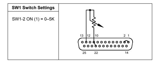
Set up for resistance programming of the output current as follows:
