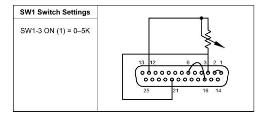
Set up for resistance programming of the output voltage as follows:
