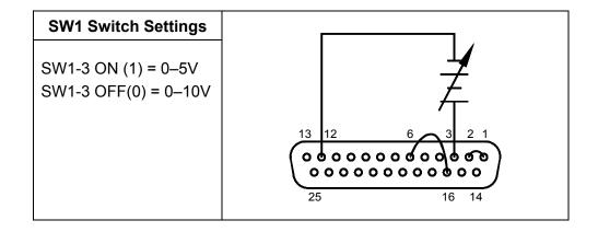
Set up for voltage source programming of OVP as follows:
