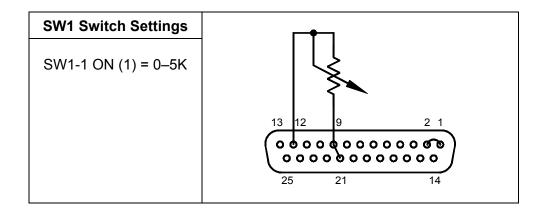
Set up for resistance programming of the output voltage as follows:
